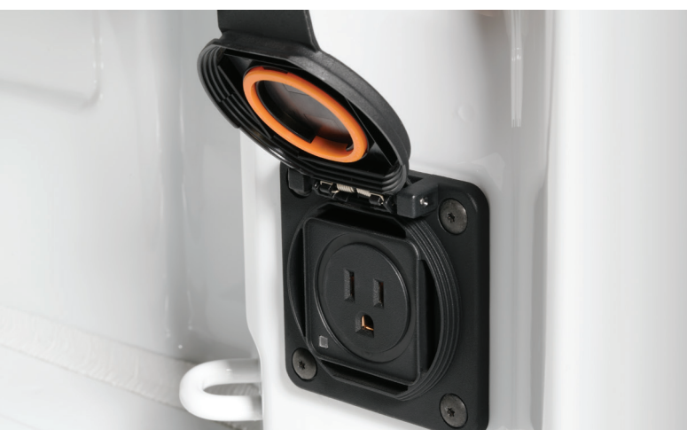
Standard 120-volt power outlet in bed
