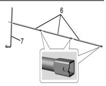
1. Assemble the wheel wrench (7) and the three jack handle extensions (6), as shown.
