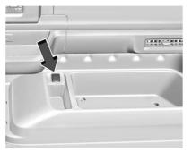
The vehicle has an accessory power outlet on the lower center stack below the climate control. Open the cover to access and replace when not in use.
