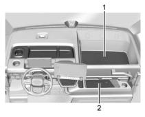
The maximum weight limit for the upper passenger side storage unit (1) is 57.7 kg (125 lb). The maximum weight limit for the lower passenger side storage unit (2) is 20.4 kg (45 lb).
