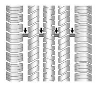
Treadwear indicators are one way to tell when it is time for new tires. Treadwear indicators appear when the tires have only 1.6 mm (1/16 in) or less of tread remaining. See Tire Inspection  $\Rightarrow$  207 and Tire Rotation  $\Rightarrow$  208.
