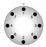
14. Tighten the nuts firmly in a crisscross sequence, as shown, by turning the wheel wrench clockwise.
