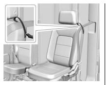
If the seat has a seat belt guide, the seat belt must be routed through the guide to properly position the shoulder belt. If the seat belt is not routed through the guide, slide the edge of the belt webbing through the opening on the guide. Be sure the belt is not twisted.
