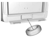
5. Tilt the tire toward the vehicle with some slack in the cable to access the tire/wheel retainer.
