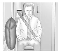
If equipped, the passenger side impact airbag is on the airbag trim cover adjacent to the jumpseat.
