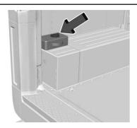
To access the inflator kit, loosen and remove the retainer.
