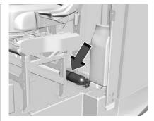
The fire extinguisher is mounted and secured with a vehicle bracket behind the driver seat.
