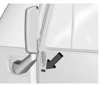
The remote key must be within 1 m (3 ft) of the door (including the rear sliding door) being opened or locked. Press the button near the door handle to open. See "Keyless Access Operation" in *Remote Key Operation*  $\Rightarrow$  7.
