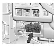
There is a fuse label in the top right pocket. Unfold it for individual fuse usage and locations. Fuse amperage ratings are shown on the fuse label. Fold label and put it back into the top right pocket.
