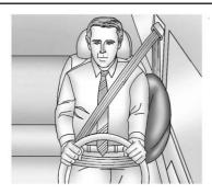
The vehicle has a seat-mounted side impact airbag for the driver in the side of the seatback closest to the door.
