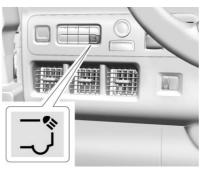
The shift lever must be in P (Park), R (Reverse), or N (Neutral) to operate the cargo lamps.
