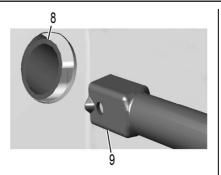
4. Insert the hoist end (9) through the hole (8) in the rear bumper and onto the hoist shaft.
