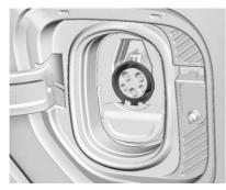
The vehicle is equipped with a charge port light. When the charge cord is plugged in, a color appears to indicate the charging status.
