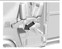
The battery is under a mat and cover in front of the driver seat on the floor.
