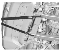
If equipped, the vehicle may have specific attachment points to be used to pull the vehicle onto a flatbed car carrier from a flat road surface. Do not use these attachment points to pull the vehicle from snow, mud, sand, or ditch.
