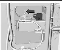
In case the door does not unlock while opening, make sure that the door is completely closed by pushing downward on the top surface of the latching cover before repeating the procedure.
