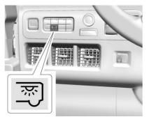
Press the button on the instrument panel to turn the cargo lamps on and off.
