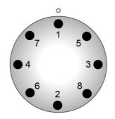
14. Tighten the nuts firmly in a crisscross sequence, as shown, by turning the wheel wrench clockwise.
