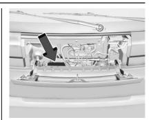
2. Remove the cover to access the Underhood Compartment Fuse Block. To open the fuse block cover, press the clips at the side and back and pull the cover up.
