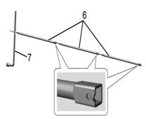
3. Attach the wheel wrench (7) and extensions (6) together, as shown.
