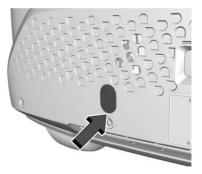
If equipped, carefully open the cover in the fascia by using the small notch that conceals the tow eye socket.
