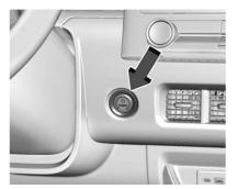
The vehicle has an electronic pushbutton start.
