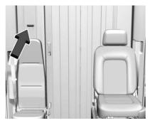
To open the sliding (bulkhead) door, unlock using the touchpad, then pull the handle and slide the door to the side until it latches.
