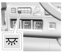
The dome lamps control is on the instrument panel.
