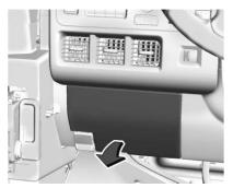
The instrument panel fuse block is on the driver side of the instrument panel, between the steering wheel and the door.
