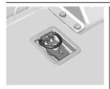
The cargo tie-downs can be used to strap cargo down and keep it from moving inside the vehicle.
