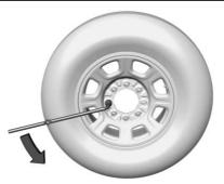
Use the wheel wrench and turn it counterclockwise to loosen the wheel nuts. Do not remove the wheel nuts yet.
