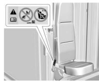
The label shown below is located on passenger side jump seat belt outboard anchor.
