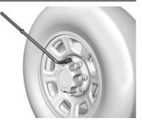
2. If the vehicle has a center cap with wheel nut caps, the wheel nut caps are designed to stay with the center cap after they are loosened. Remove the entire center cap.
