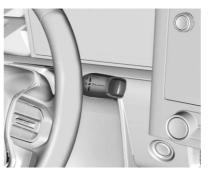
The vehicle uses an electric drive unit. The shift pattern is displayed on the front of the shift lever. The selected gear position will illuminate red on the shift lever, while all others will be displayed in white. If the shift is not immediate, as in very cold conditions, the indicator on the shift switch may blink until it is fullu engaged.
