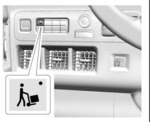
To activate Delivery mode, press the Delivery mode button. An indicator light will illuminate when Delivery mode is active.
