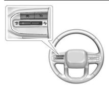
S : Press to turn the system on or off. The indicator turns white on the instrument cluster when ACC is turned on.
