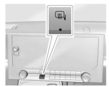
Press the button located below the infotainment display to activate the heated mirrors. The indicator light will illuminate when active.
