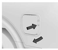
3. Unlatch the DC charging dust cover and lower it fully.
