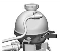
4. If the coolant level is not visible or needs to be adjusted within the reservoir, contact your dealer.
