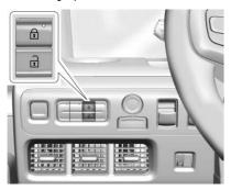
**•** : Press to lock all doors. The indicator light in the switch will illuminate when locked.
