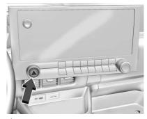
▲ : Press this button to make the front and rear turn signal lamps flash on and off. This warns others that you are having trouble. Press again to turn the flashers off.
