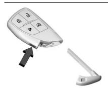
The mechanical key inside the remote key is used for the rear sliding door.
