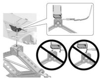
Ensure that the jack lift head is centered on the front or rear jacking pad. If equipped with a pin on the jack lift head, the pin must fit into the center of the hole in the jacking pad.
