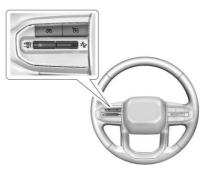
S: Press to turn cruise control on or off. A white indicator light comes on in the instrument cluster when cruise control is turned on.
