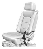
Move the lever up or down to raise or lower the seat.
