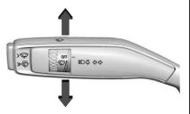
Move the lever all the way up or down to signal a turn.
