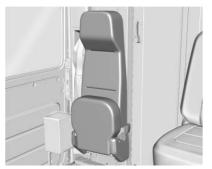
To use the jump seat, pull down on the seat cushion until the seat is in place. To store the seat, return the seat cushion to the upright position.
