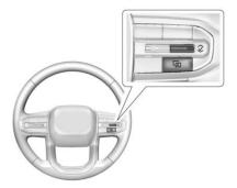
Use the right steering wheel control to open and scroll through the different items and displays
