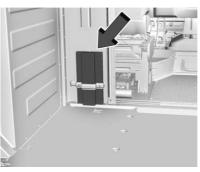
If equipped, warning triangles are located behind the driver seat, stowed in a bulkhead area. To remove, lift them out of the storage bracket.
